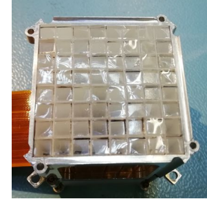
top side Silicone pads on CsI crystals
