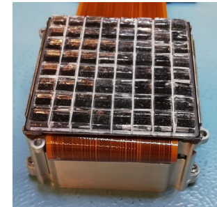
bottom side Silicone pads on SDD
