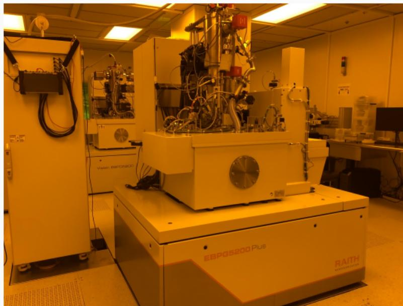
**Figure:** RAITH EBPG 5200 & 5200+ 100 keV EBL tools at PSU
