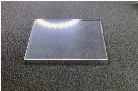
CsI (Tl) scintillator – 5x higher yield than BGO (lower energy threshold)
