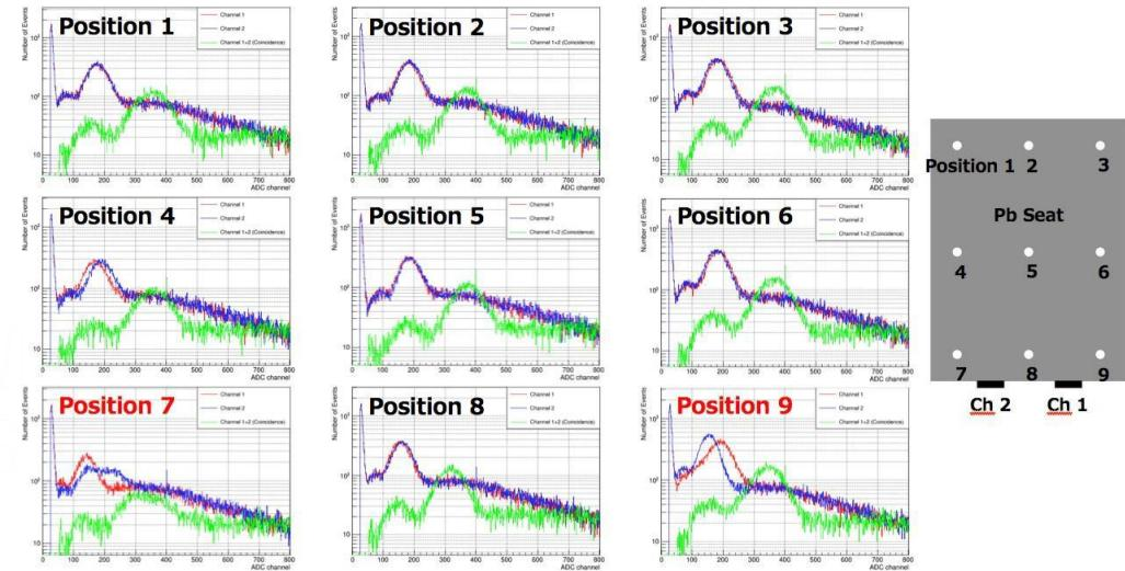
variation of detector response for gamma source at different positions
