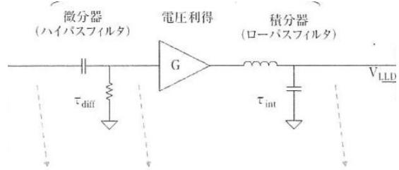
final 2-stage amplifier ( $R_1C_1=3.3\text{ ms}$  decay,
