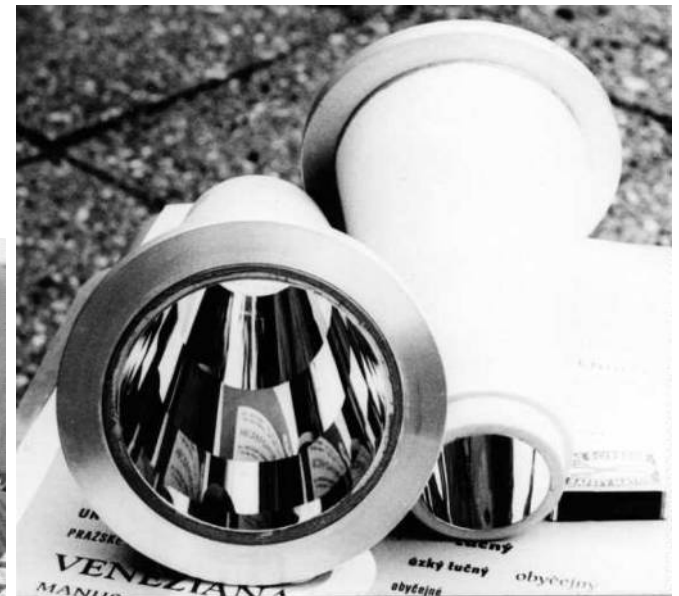
Two identical mirrors (large hyperbolas) of the RT-4M mirror array (Ni surfaces), 1981.
