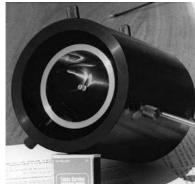
The four mandrel used for the manufacture of X-ray mirror nested array for the RT-4M soft X-ray telescope (Glass ceramics Sital). Flown onboard the space station Salyut 7 in 1981.
