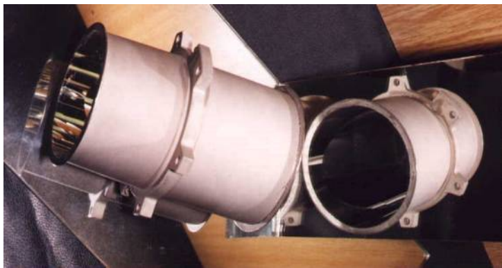
Replicated Wolter - 1 X-ray mirrors of the KORONAS satellite (aperture 80 mm), 1989
