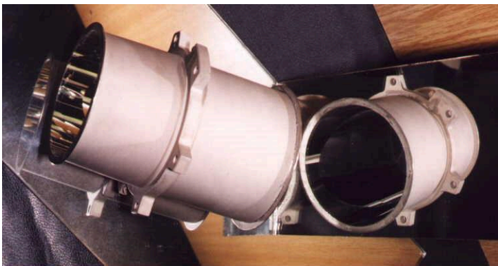
Replicated Wolter - 1 X-ray mirrors of the KORONAS satellite (aperture 80 mm), 1989
