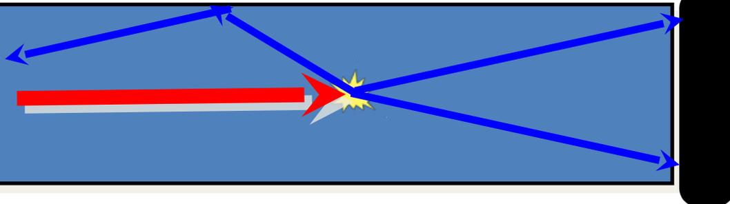
$\gamma$ -ray events: scintillation light readout by both SDDs Position reconstruction possible using the two signals
