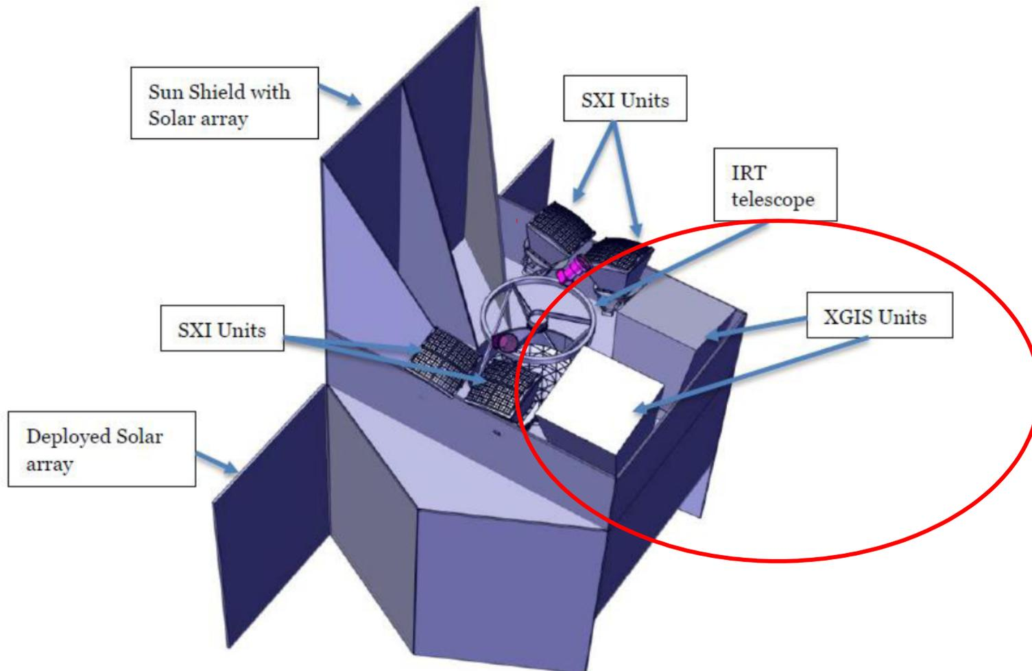
Figure 2: THESEUS spacecraft current design and payload accommodation
