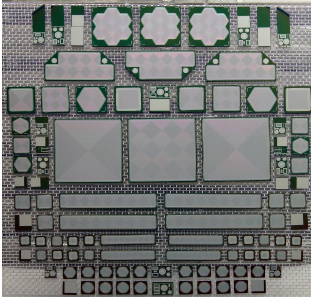
Silicon Drift Detectors (SDD) from REDSOX project (INFN) realized at Fondazione Bruno Kessler (FBK Trento)
