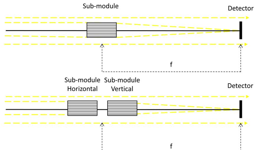
**Fig. 1:** Arrangement comparison of 1D (top image) and 2D (bottom image) LE optics
